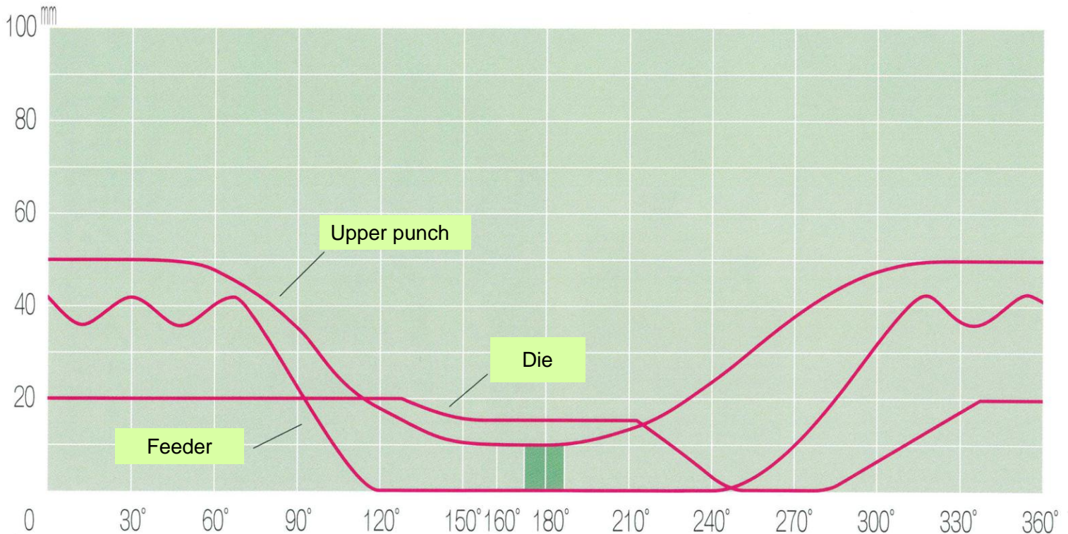
PB-1 CAM DIAGRAM
